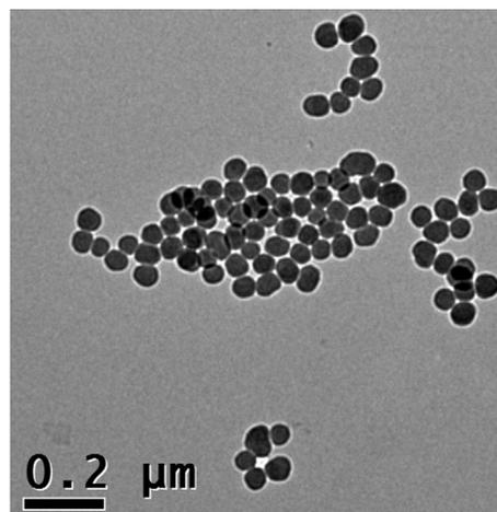
**Fig. 1.** Representative TEM image of tested SiNPs. All particles were near-spherical in shape, and had good monodispersity. The scale bar, 0.2  $\mu\text{m}$ .
